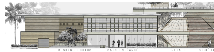
BESIDE THE LARGE OVERHANGS, THE PROTRUDING UPPER FLOORS NATURALLY SHADED THE LOWER FLOOR MAIN ENTRANCE AS WELL.
