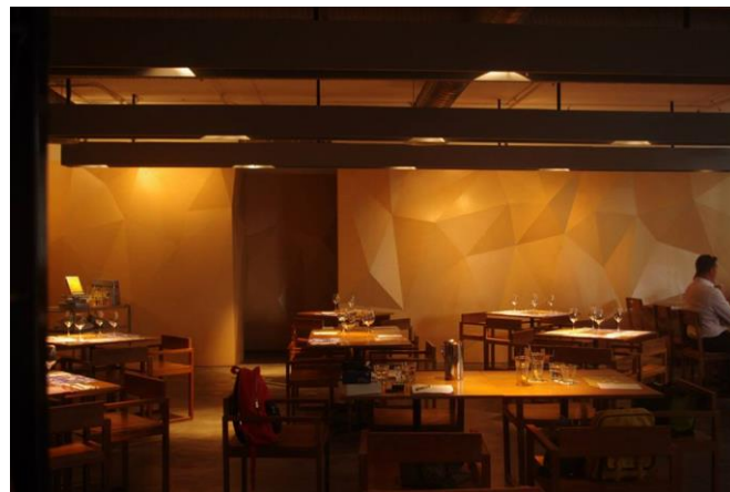
Figure 3.3.2.1: Faceted wooden walls are found along the main dining area which act as sound insulators
