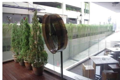
Figure 3.3.1.2.4: Stand fan which is main noise contributor at Room 5
