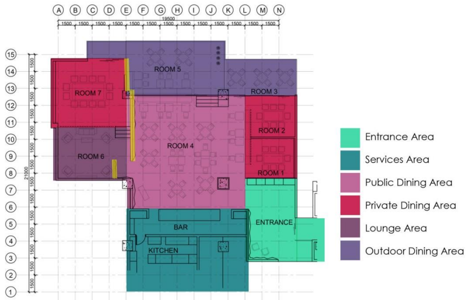
Diagram 3.4.6.2.1: Yellow line indicating divider between public dining area and private dining area
