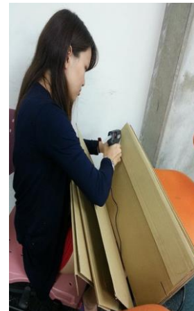
Figure 39 Connecting piece by piece using hot glue gun.
